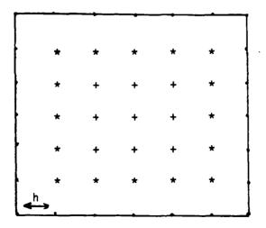
Figure 2.1. The uniform discretization of R.
