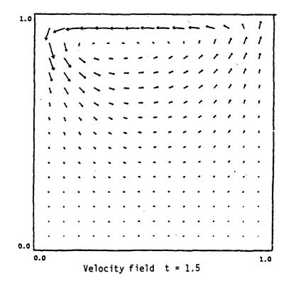
Figure 5.6 Discrete solution of the time dependent Navier Stokes equation at Reynold's number 200.
