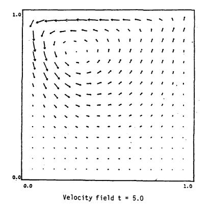
Figure 5.7 Discrete solution of the time dependent Navier Stokes equation at Reynold's number 200.
