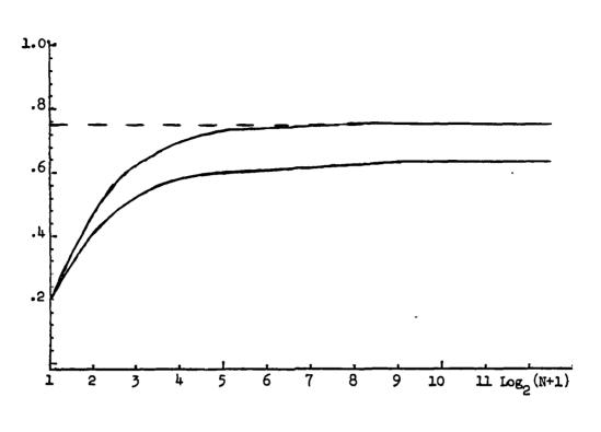
Figure 3.1. The largest singular value as a function of  $\log_2(N+1)$  (below), compared with the corresponding Gershgorin bound (above).
