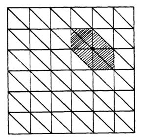
Figure 2.2. Finite element triangulation corresponding to the 13-point difference stencil.
